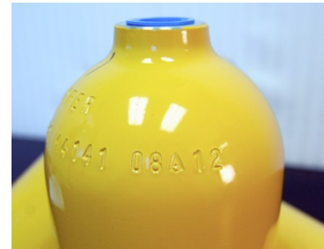
Figure 41: Hydrostatic Test Date
