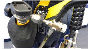
After EEL airline, the exposed ends should be protected during cleaning and storage. Inspect the hose for cracks, blisters and signs of wear.
